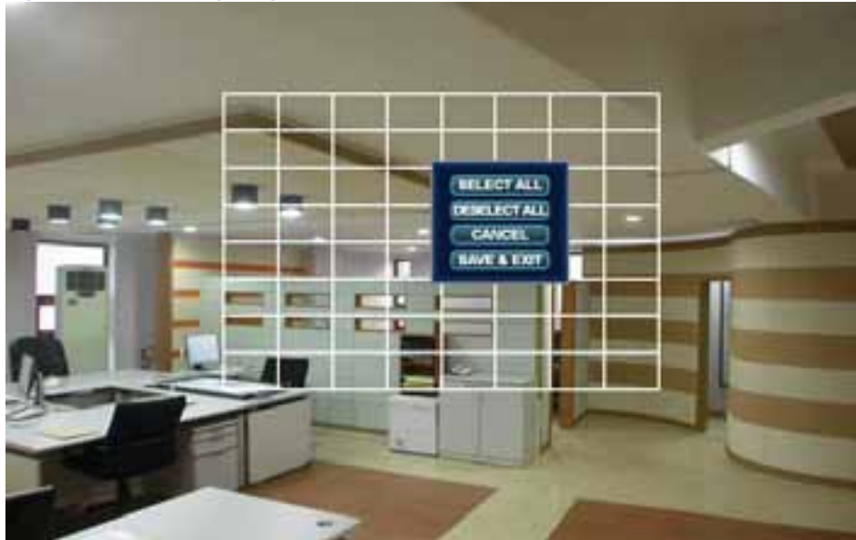
Figure 2-24 Configuring the Motion Sensor Area
