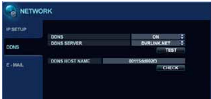
Figure 2-49 DDNS Setup Window
