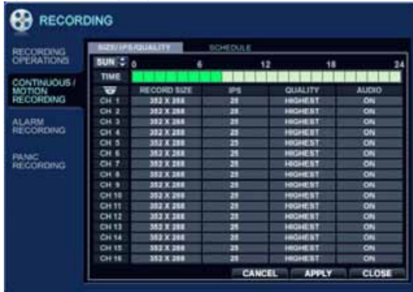
Figure 2-60 Configuring SIZE/IPS/QUALITY Time Bar
