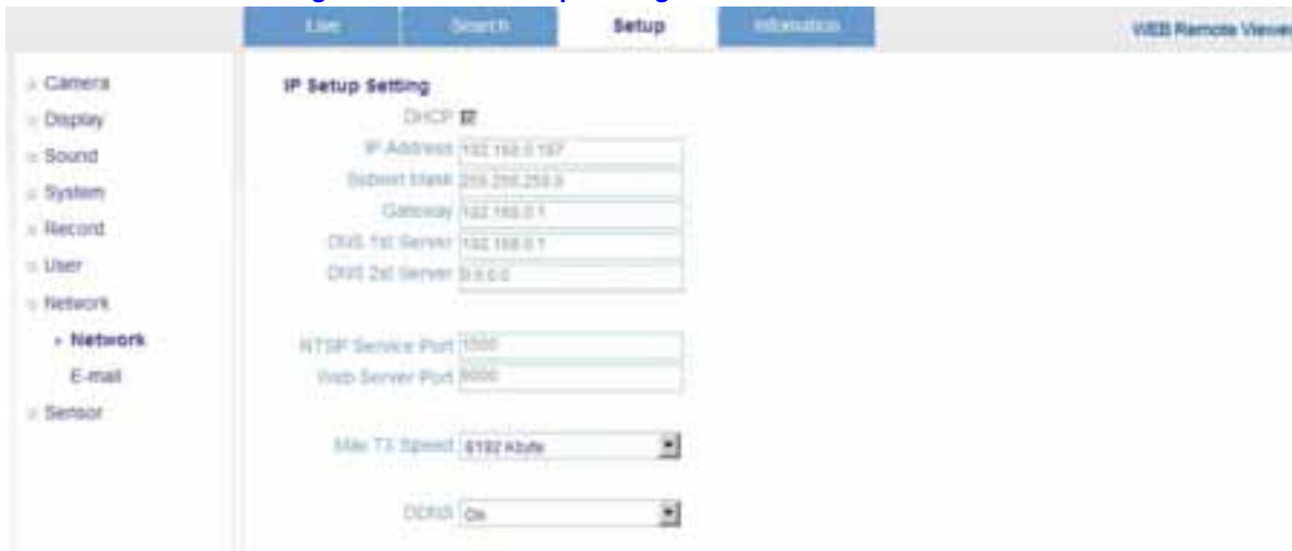
Figure 4-20 IP Setup Setting Window
