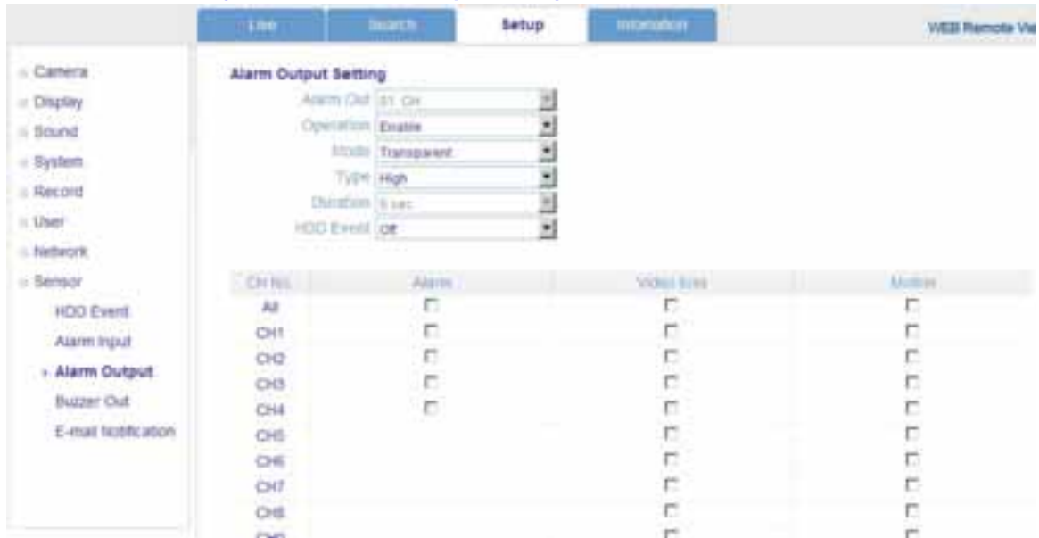
Figure 4-22 Alarm Output Setting Window
