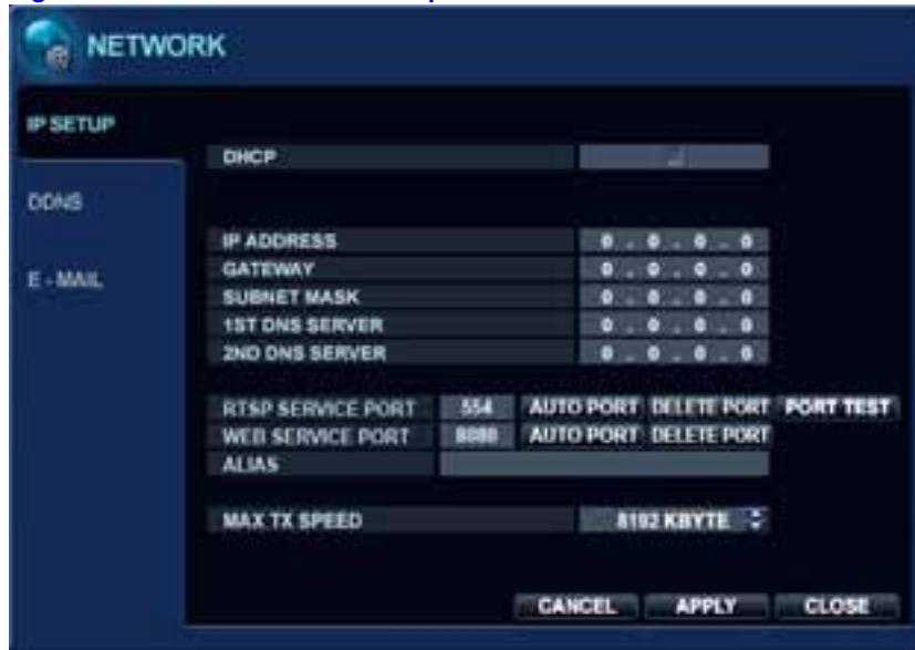
Figure 2-48 IP NETWORK Setup Window
