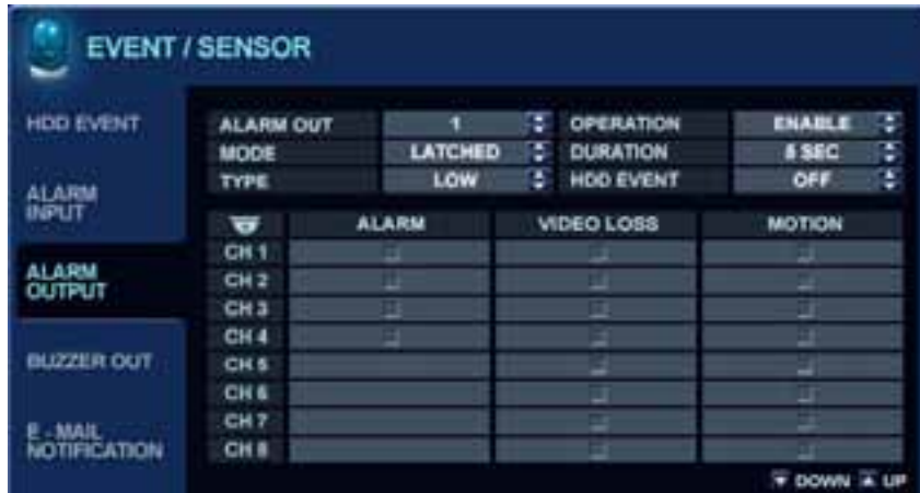
Figure 2-53 ALARM OUTPUT Setup Menu
