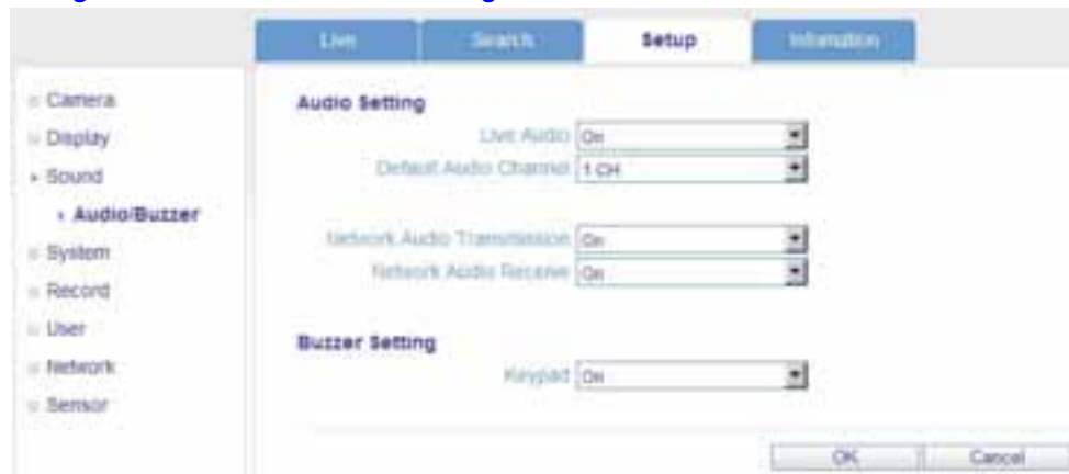
Figure 4-16 Audio/Buzzer Setting Window
