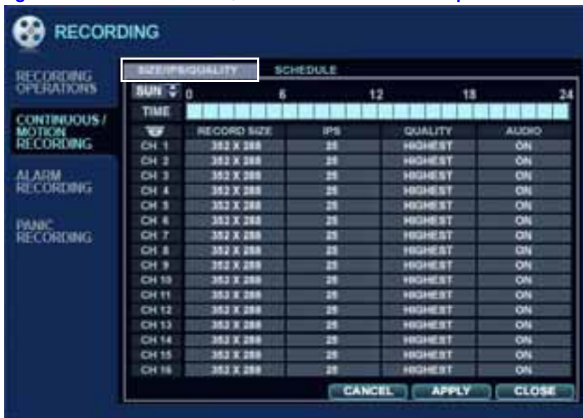
Figure 2-59 CONTINUOUS/MOTION RECORDING Setup Window
