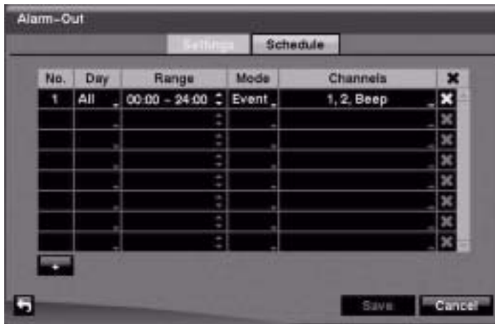
Figure 3-40 Alarm-Out Schedule Screen
